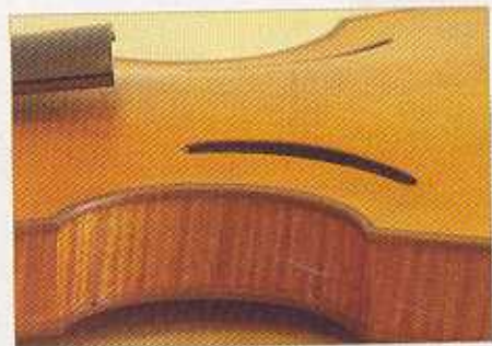
FIG. 1: The simple, gamba-like corners on this Joseph Curtin ultralight violin stay well out of the player's way, while the hardwood edges provide an added measure of durability.
