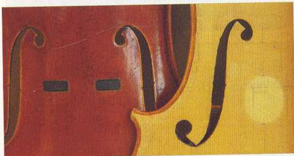
FIG. 5: Hardwood veneers under the bridge feet and on the inside of the top beneath the soundpost prevent damage in these two highly vulnerable areas.
